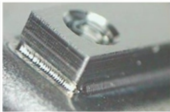
Inside Corner Seam Welding
